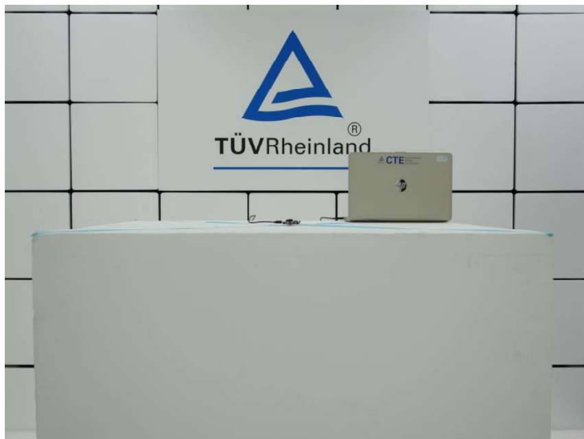
Photograph 1: Setup for Radiated Emission (Front View)
